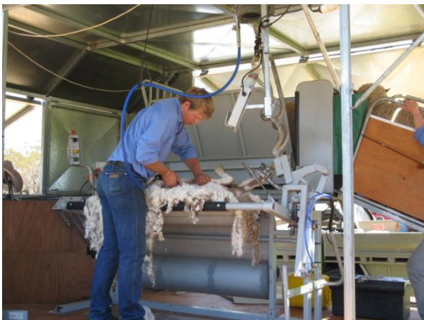
David Willersdorf demonstrates the ram shearing trailer primarily set up to reduce handling risks.
